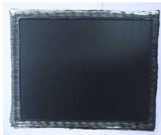
Figure 5. Representative hybrid composite laminate with carbon nanotubes, fabricated through Resin Film Infusion. [Color figure can be viewed in the online issue, which is available at wileyonlinelibrary.com .]
